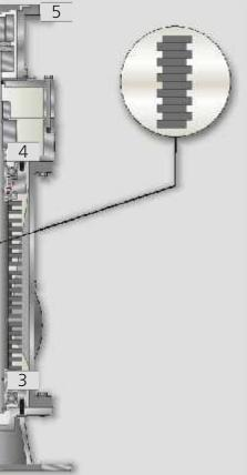
6 In-line Version Product inlet and outlet are positioned on the same level. The NETZSCH twin shaft macerator can be directly connected into a horizontal pipeline or to a pump inlet of a NEMO<sup>®</sup> pump or a NETZSCH TORNADO<sup>®</sup> industrial rotary lobe pump, where flange is set at 90°.
